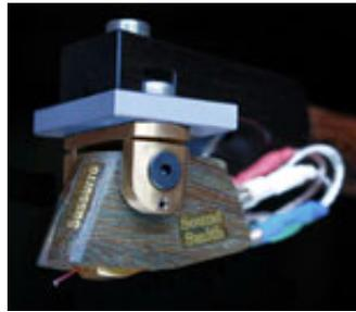
10. The Sussurro moving-iron cartridge from Soundsmith also resides in a wooden body, employs a nude contact line diamond stylus, and weighs 8.79 g.
